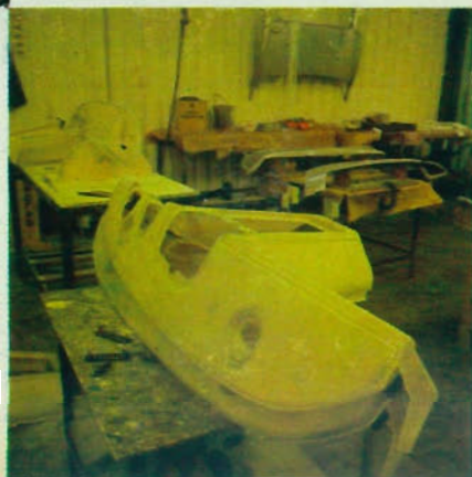
Left: Line up of a day's production. These are Interceptor Mark 1 models, photographed before the change to Mark 2 specification. Right: With a long background of glass-fibre experience, Jensen use this material for interior panels like the facia and console
