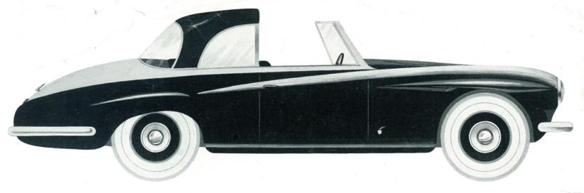
Designed and constructed on sleek, wind-cheating lines. Excellent visibility is afforded through the straight laminated glass windscreen which is positioned as near to the driver as possible to avoid interior fitting reflections. Opening type ventilator windows are fitted to the front of the doors and both the door and quarter windows lower completely. A large window is fitted in the rear of the hood.
