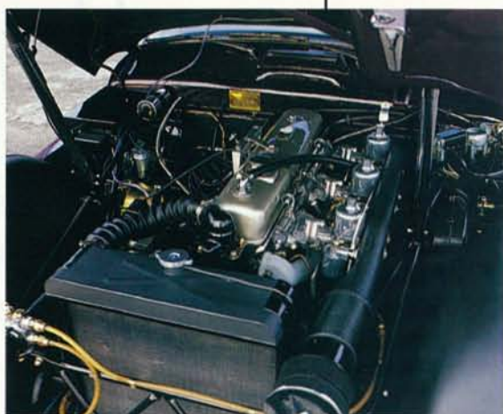
Above: bonnet catch. Left: Motorola radio with 'Jensen' sign. Below: DS5 engine fitted with three SU carburetors
