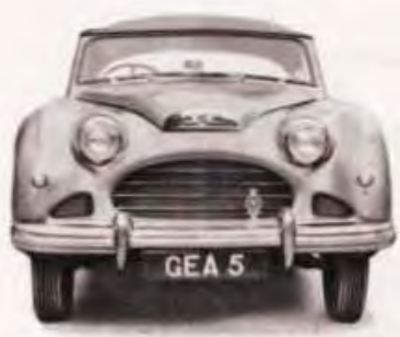
The wide shallow radiator grille is a prominent feature of the distinctive full-width front. The small side grilles allow air to flow over the brake drums.
