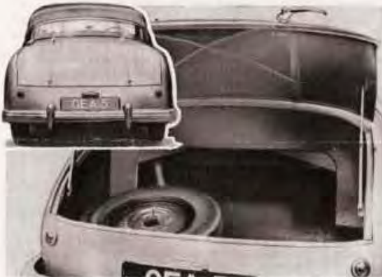
Although the large tail locker houses the spare wheel it also provides very generous luggage space. The lid is of light weight and is braced by tubular framing; it is supported at each side. Excellent rearward visibility is given by the transparent lower section of the head.
