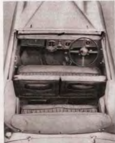
The bench-type front seat is wide enough for three, and the squab is divided, each half folding forward to give easy access to the rear seat. Instruments are neatly grouped in the centre of the leather-covered fascia, with the rev counter in front of the driver. Large wells provide ample leg-room for the rear passengers.
