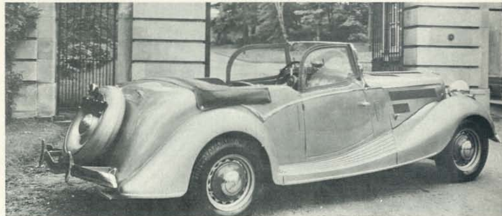
Clark Gable brought home this 1936 Jensen. Lengthened wheelbase shows up in stretched fenders. Jensen used unmodified Ford suspension, brakes, running gear. Columbia 2-speed was standard.
