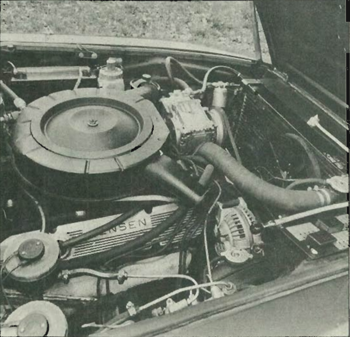
Above: From the 1967 Autotest of the Interceptor, featuring the Italian-designed steel bodywork Below left: Well-equipped dashboard of Interceptor Mk II Below right: Earlier Interceptors were fitted with this 6,276 c.c. engine which produced 325 bhp Bottom left. Interceptor III in convertible guise Bottom right: Snug rear seats provide excellent sideways location. Note neat hood cover
