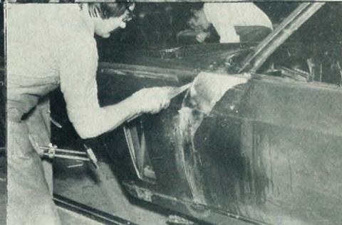
Heart of the Interceptor chassis is the substantial twin-tube construction with one member functioning as the servo reservoir; pressed steel panels are bought out but they are all jig-welded together at Jensen's factory. A steel "monocoque" is welded to the tubular members, bottom left; top right, a section of the convertible's tail. There is still room for craftsmen at Jensen, witness planishing the door and lead-filling for constant door fit
