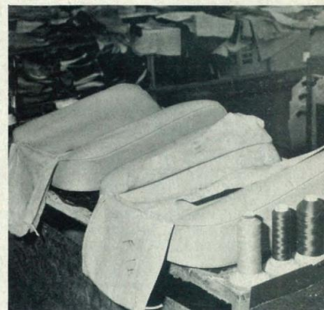
At the end of the interior trimming line the wiring looms are fitted having been made up alongside the track. Seats are hand made upstairs and some six hides are used in each car
