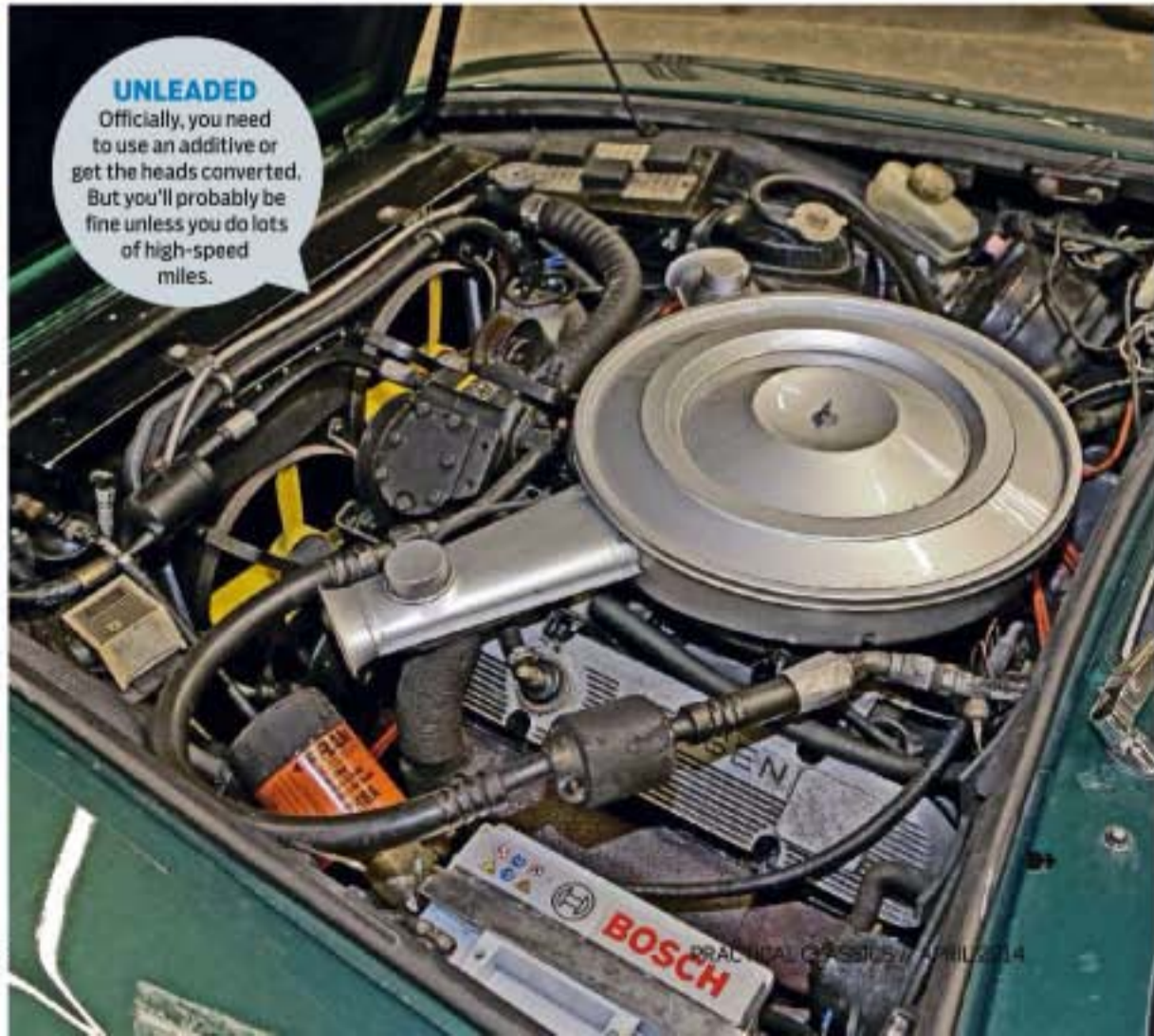
Fuel hoses get cooked by the exhaust, then perish with predictable results.
