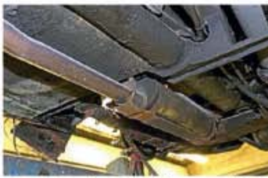
The twin-pipe exhaust system features multiple sections that often don't fit together very well.
